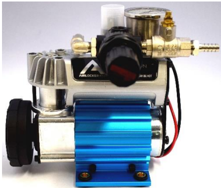
Figure 2-2 Air compressor feeding the Ramsay valve with compressed air
